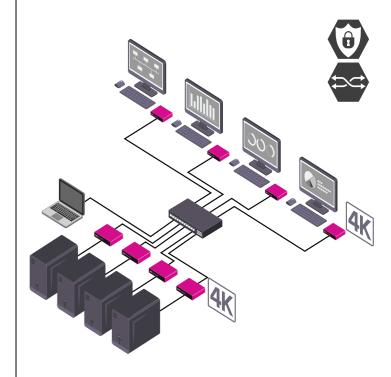
Pathfinder 500 and 800 series endpoints can be integrated into a large matrix system using standard networking switches. Switching between PC's is easily achieved using an On Screen Display (OSD) menu, user definable hot keys or with our intuitive Pathfinder Control software.
